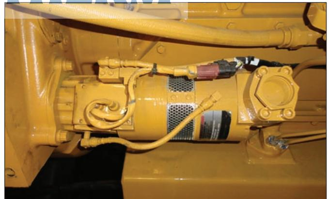
TurboStartTwo on Caterpillar C32 engine.
